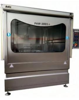
**Stainless Steel** 200x175x200 cm (Machine Dimension) **Basket Diameter 135 cm** Loading Height Max. 70 cm Loading Weight Max. 650 kg Tank Capacity 300 lt. **Pneumatic Door Automatic Cleaning Rotating Basket Reducer High Pressure Cleaning 6 bar High Pressure Cleaning Nozzles Water Temperature Control** Water Heater 90 Deg. **Discharge Station Cleaning Timer Control** Oil Skimmer **Loading Vehicle**
